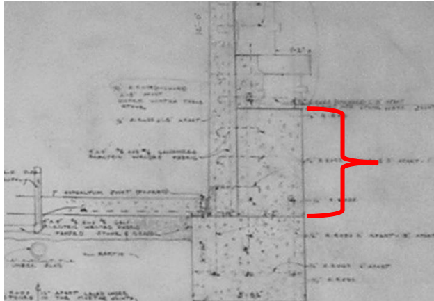
Figure 315. Detail from original construction drawings of the west reservoir at the Bridge Complex showing a cast-in-place concrete curb (bracketed area) that bears on the concrete foundation and covers the lower portion of the reservoir walls. (Source: Caldwell Archives at the Dubuque Museum of Art)
