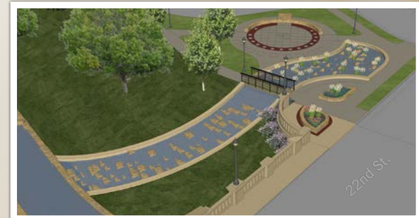
The 22nd St. spillway provides a way for floodwater to flow from a higher elevation, the street, to a lower elevation, the creek, in such a way as to prevent erosion of the surrounding soils.
