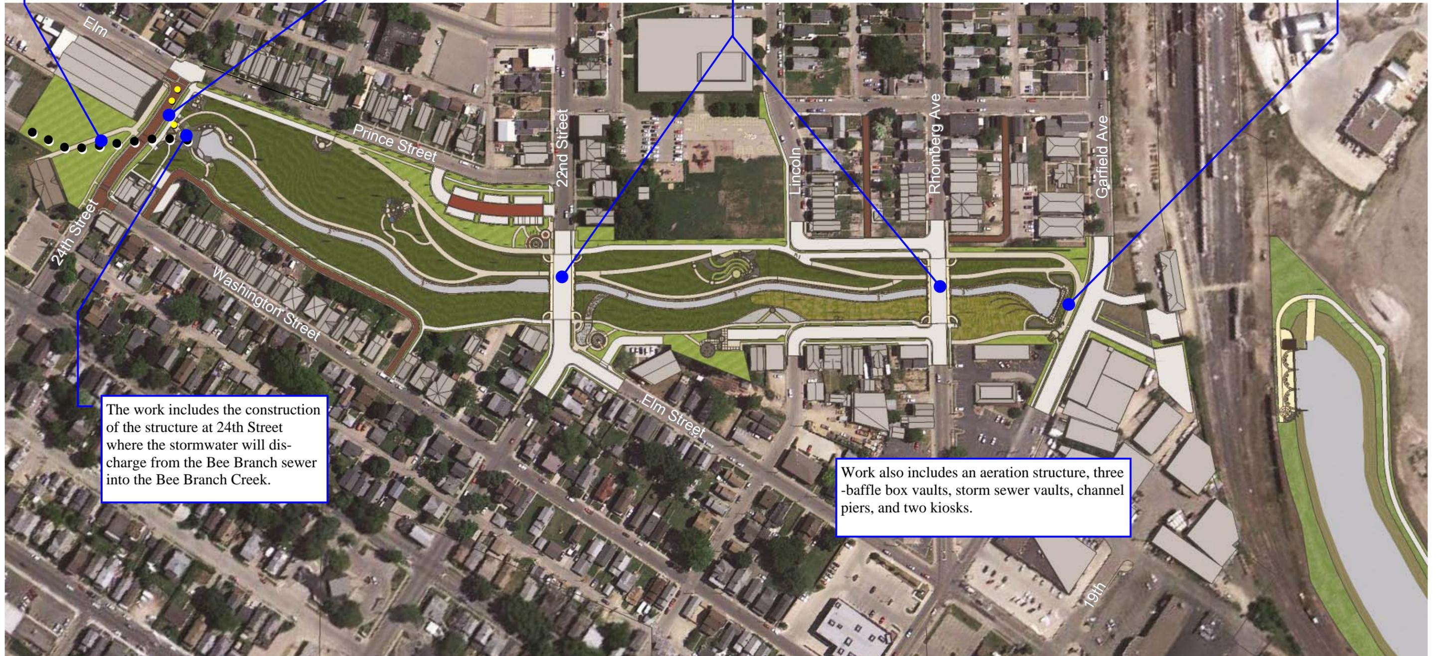
The work includes the construction of the structure at 24th Street where the stormwater will discharge from the Bee Branch sewer into the Bee Branch Creek.
