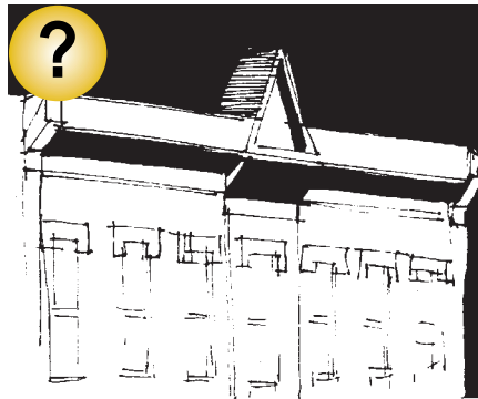
A simplified interpretation is also appropriate for a replacement cornice if evidence of the original is missing.
