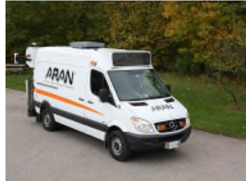
Pavement Scanning Van – Measures Smoothness and cracking
